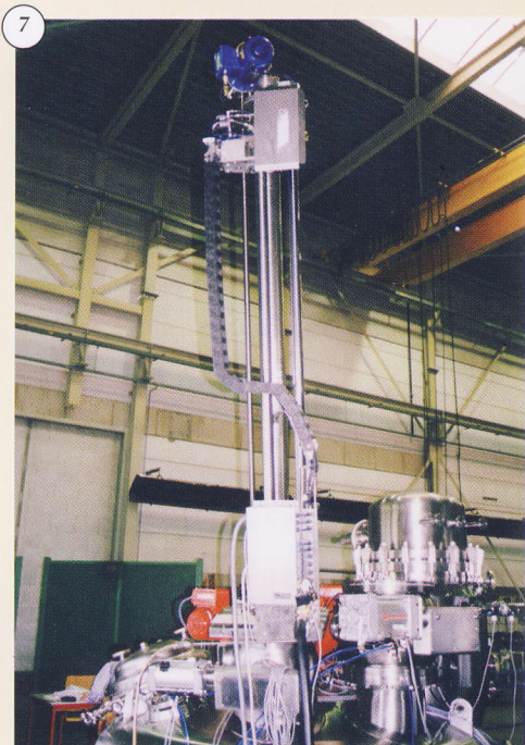
4 Dryer, as it looks after production, with residues of active substance, prior to the CyberjEt® carrying out nitrogen-based product recovery.
