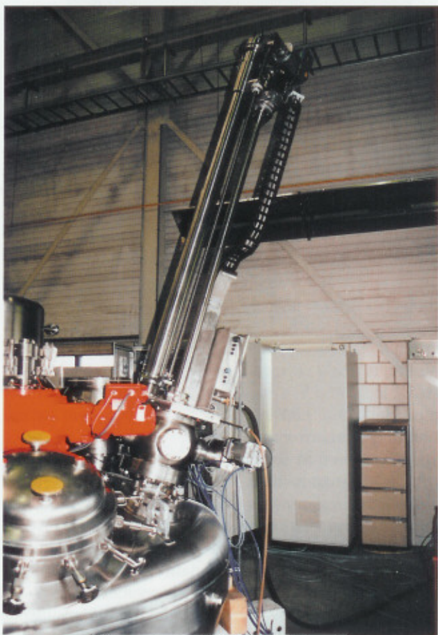
The patented CyberjEt is utilised for the cleaning of tanks
