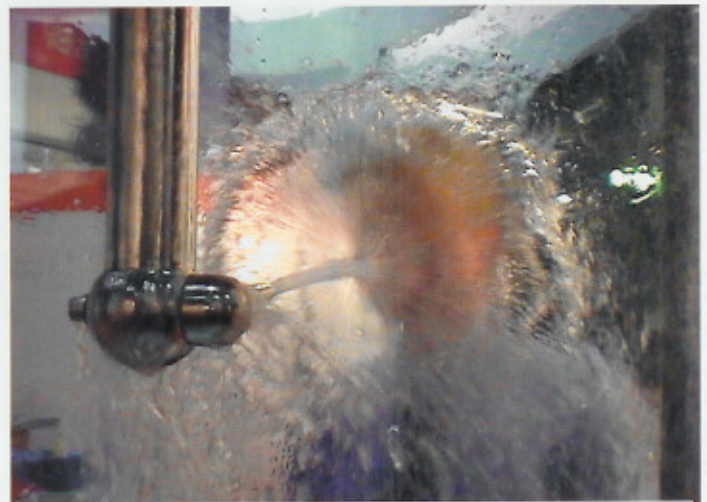
The movement of the rotating spray nozzle is able to adjust the cleaning medium in the tank through a programmed control
